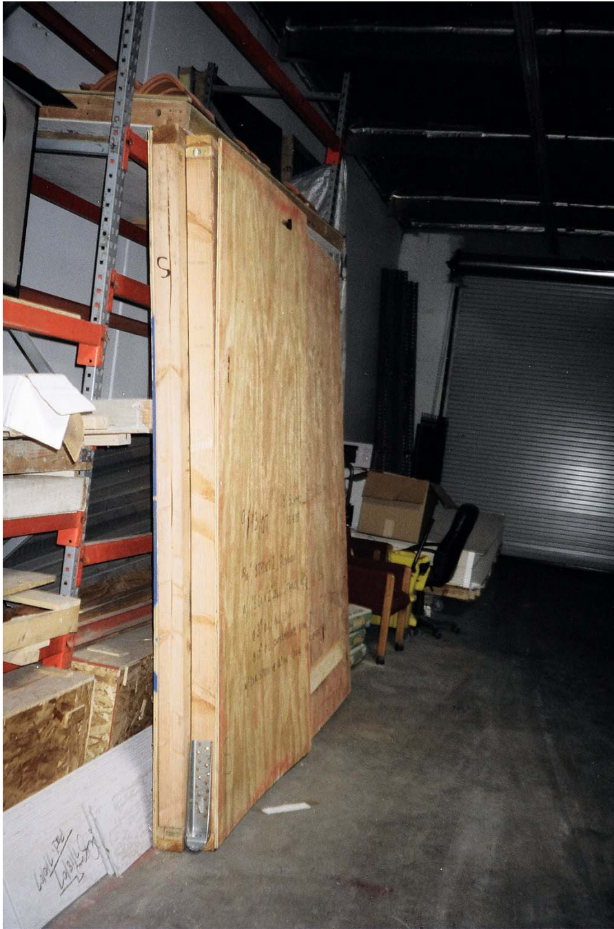
Photo 1: View of 16 ga. stapled shear wall after test showing plywood loose at top and bottom with staples sheared at surface between back of plywood and face of studs.
